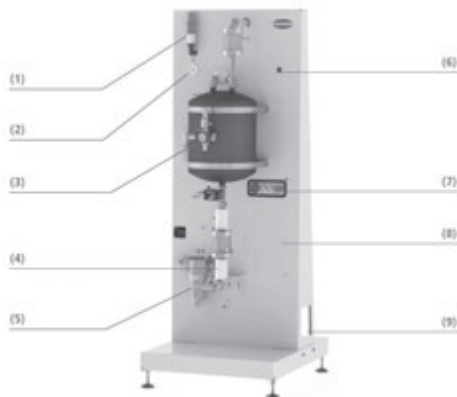
Systemaufbau Vacuum Operation Center VOC
